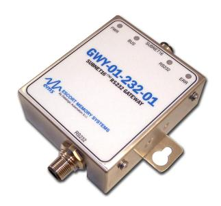
The EMS Gateway supports Subnet 16<sup>™</sup>, a subnetwork of up to sixteen EMS RFID controller/antenna stations. Subnet16 thus concentrates many read/write devices into one convenient connection point for host networks in the factory or enterprise.
